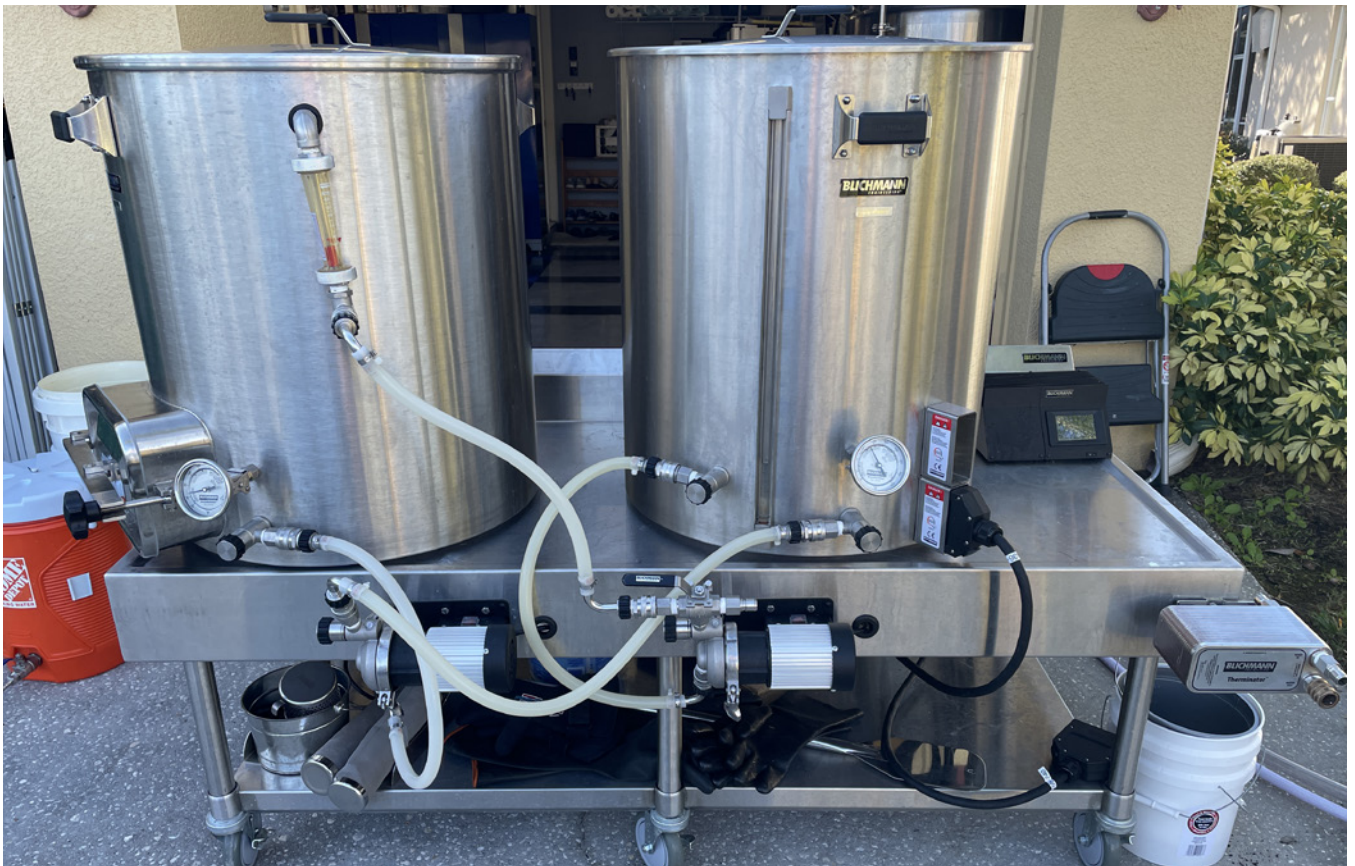
The Fairgate Brewing system is a 1-BBL two-vessel electric Blichmann BrewEasy™ Pro system with a custom manway for easier cleanup of the spent grains.
